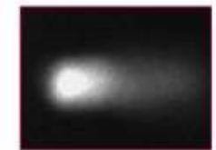
Output from fibre, incident directly onto CCD (no lens).
